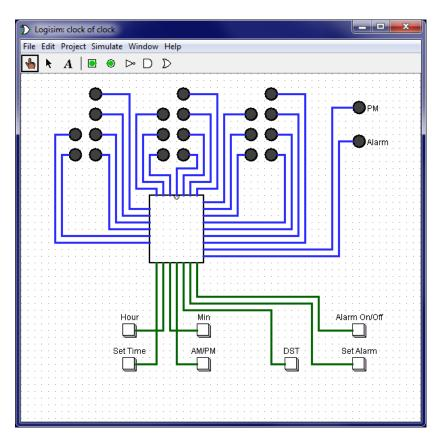
This circuit shows Buttons and LEDs required for all Milestones below; you only need to provide those required at each Milestone. Note that Logisim only allows you to press one button at a time.
