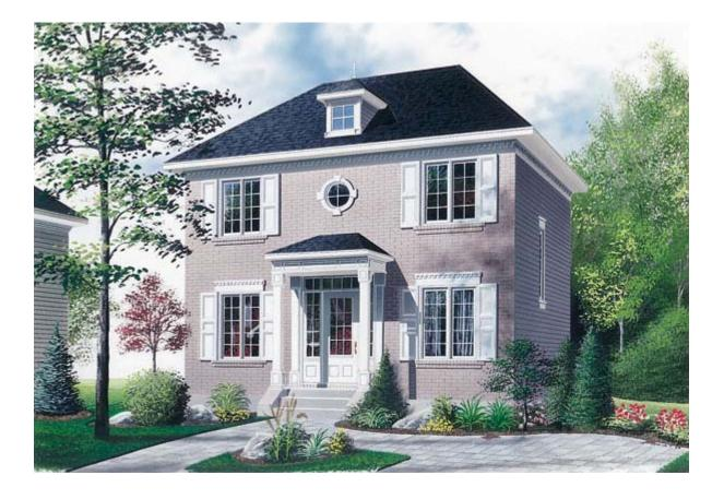
Number of Bedrooms: 3 Number of Bathrooms: 2.0 Width of House: 27 feet Depth of House: 27 feet Architectural Style: Colonial Exterior Wall Structure: 2x6 studs Roof Framing: Truss Roof Peak: 28 feet from Front Door Floor Level Roof Load: 40 p.s.f.
