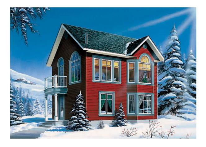
Number of Bedrooms: 2 Number of Bathrooms: 2.0 Width of House: 22 feet Depth of House: 26 feet 1st Floor Plateline: 8'0 Architectural Style: Colonial Exterior Wall Structure: 2x6 studs Roof Framing: Truss Primary Roof Pitch: 10:12 Roof Peak: 28 feet from Front Door Floor Level
