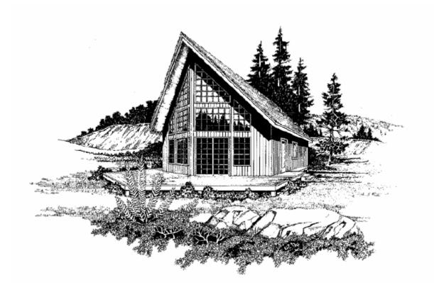
Number of Bedrooms: 1 Number of Bathrooms: 1.0 Width of House: 24 feet Depth of House: 38 feet 1st Floor Plateline: 8'0 Foundation Type(s) available for this plan: Crawlspace Architectural Style: Vacation Exterior Finish: Siding Exterior Wall Structure: 2x6 studs Roof Framing: Stick Primary Roof Pitch: 12:12
